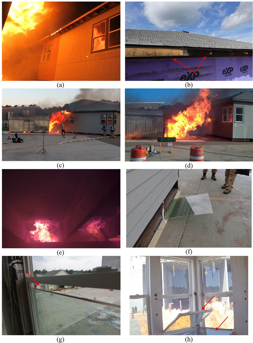
Fig. 6 Damage observed on the target building in these experiments corresponds to the destroyed category: a–b ignition of the fascia board, c ignition of the eave, d–e ignition of the siding and flame penetration in to the attic through the vents, f–g failure of the first and second window pane, h window sash failing inwards
