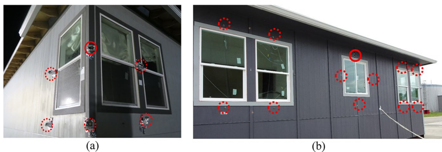
Fig. 3 Sensor layout for tests with target building orientations of (a) 45° and (b) 0°. Data from the sensor outlined in solid lines is used in the discussion section
